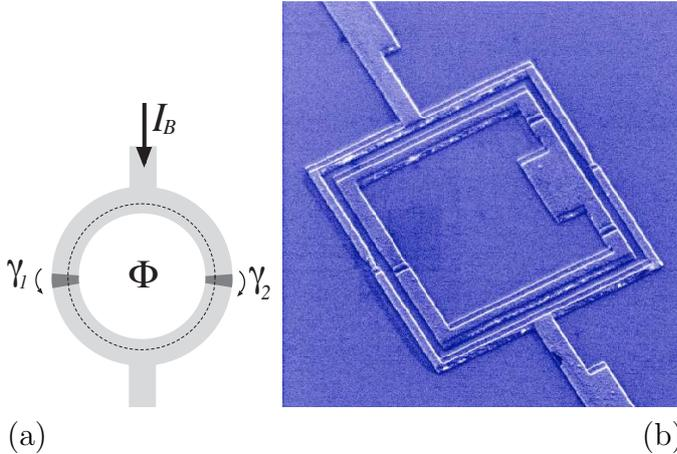
Figure 2.4: (a) Schematic representation of a superconducting quantum interference device. Two junctions described by the gauge-invariant phase difference  $\gamma_1$  and  $\gamma_2$  enclose the flux  $\Phi$ . (b) Configuration of the original Delft flux qubit with a surrounding readout SQUID. The qubit state influences the critical current of the SQUID [75]. Image from TU Delft.
