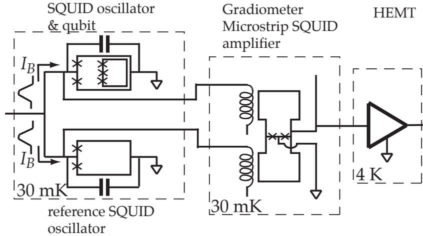
Figure 5.5: Circuit diagram for SQUID oscillator and qubit, along with reference SQUID oscillator, dual-input gradiometer microstrip amplifier and a cryogenic High Electron Mobility Transistor (HEMT). Dashed boxes indicate different chips and/or different temperatures.
