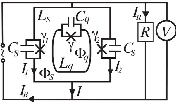
Figure 3.1: Simplified circuit consisting of a qubit with one Josephson junction (phase  $\gamma$ , capacitance  $C_q$  and inductance  $L_q$ ) inductively coupled to a SQUID with two identical junctions (phases  $\gamma_{1,2}$ , capacitance  $C_s$ ) and inductance  $L_s$ . The SQUID is driven by an AC bias  $I_B(t)$  and the voltage drop is measured by a voltmeter with internal resistance  $R$ . The total flux through the qubit loop is  $\Phi_q$  and through the SQUID is  $\Phi_s$ .
