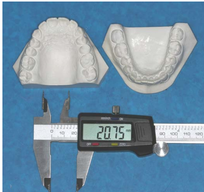
Fig 10 : Instrument for dental cast measurement : an electronic digital caliper.
