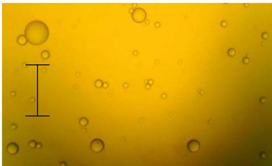
**Fig. 67.** Light microscopy analysis of components inducing turbidity in placebo syringes after ultrasound stress. Comparing this picture to the image of droplets in silicone oil emulsions verifies the siliconic nature of the particulate matter in placebo syringes; scale bar represents 100  $\mu\text{m}$ .
