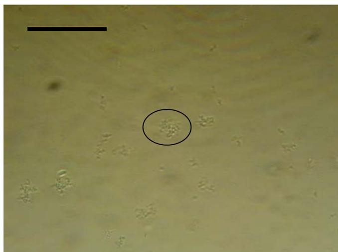
**Fig. 102.** Light microscopic analysis of a vial volume revealing visible particulate matter, highlighted by black circle (scale bar represents 100  $\mu\text{m}$ ).
