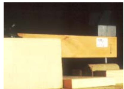
Image 62, sketch and image for the experiment set-up of the scratch test on conditioned column samples. The soil columns are approximately 5cm longer. The scratch nail made out of steel has a 2.5mm diameter and is abraded to a round cone with a 53° degree acute angle. It is upright to the sample flanks and is pressed with 1.7\text{N} \pm 0.05\text{N} weight on the sample. With the pull string, the wooden beam with the scratch nail is moved with constant speed of about 0.025 m/s across the sample.
