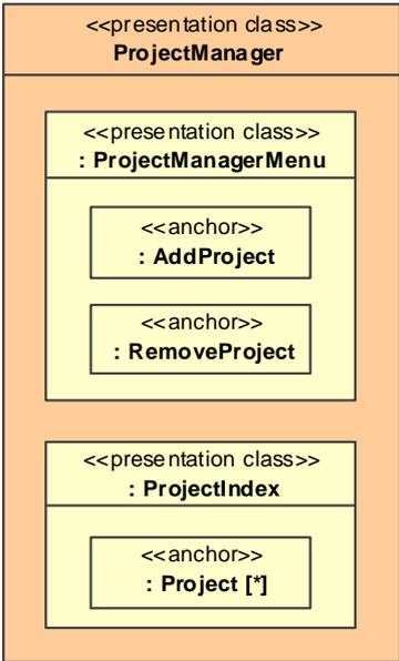
**Figure 65.** Automatically derived presentation classes for the navigation class *ProjectManager*, menu *ProjectManagerMenu* and index *ProjectIndex*
