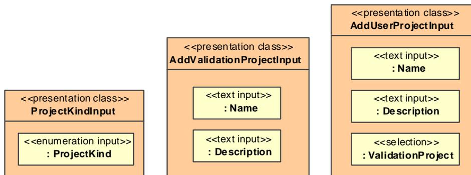
Figure 128. Automatically derived presentation classes for the process classes *ProjectKindInput*, *AddValidationProjectInput* and *AddUserProjectInput* of process *AddProject*
