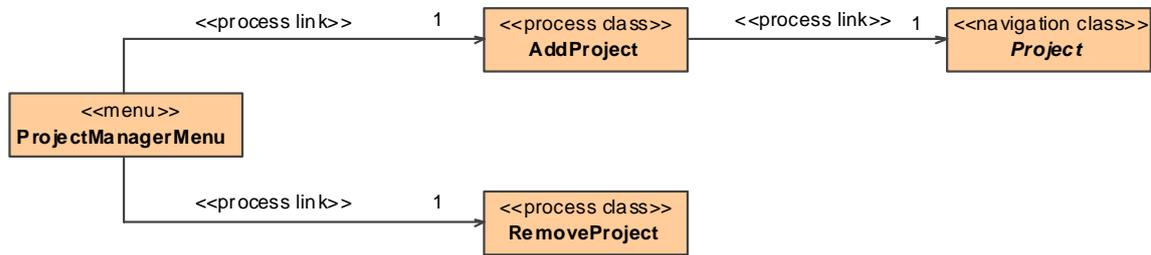
Figure 108. Automatically derived process classes and links for content class *ProjectManager*
