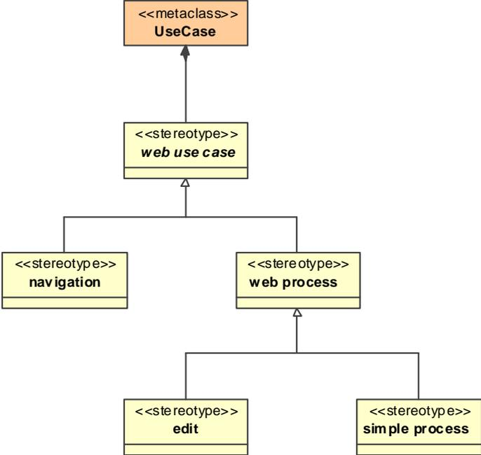
Figure 156. UML Profile for requirements modeling
