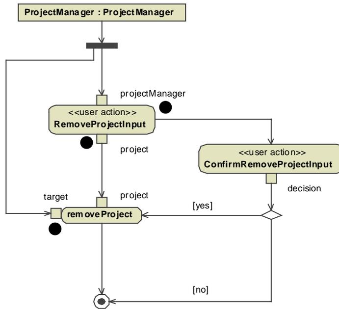
Figure 145. Token flow when executing process *RemoveProject* – step 3
