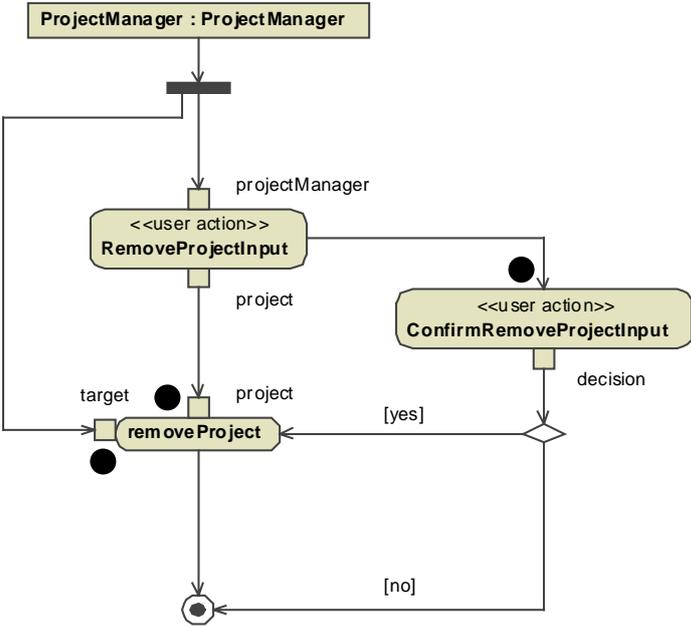
Figure 146. Token flow when executing process *RemoveProject* – step 4
