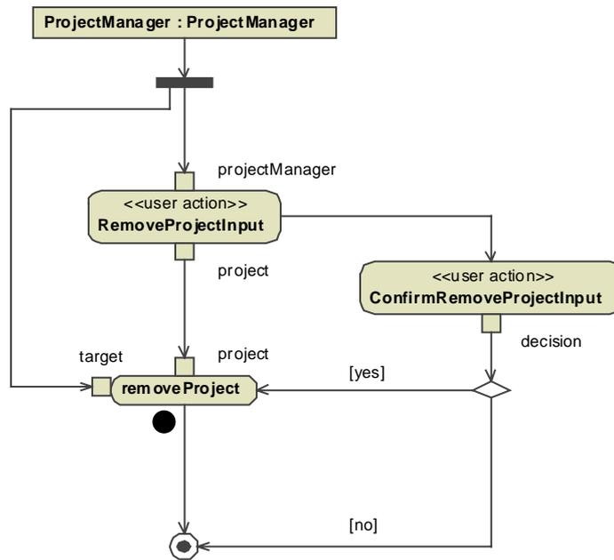
Figure 149. Token flow when executing process *RemoveProject* – step 7
