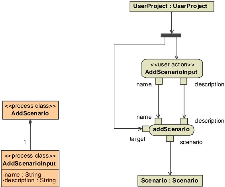
Figure 117. Automatically derived process data and flow for simple process *AddScenario*
