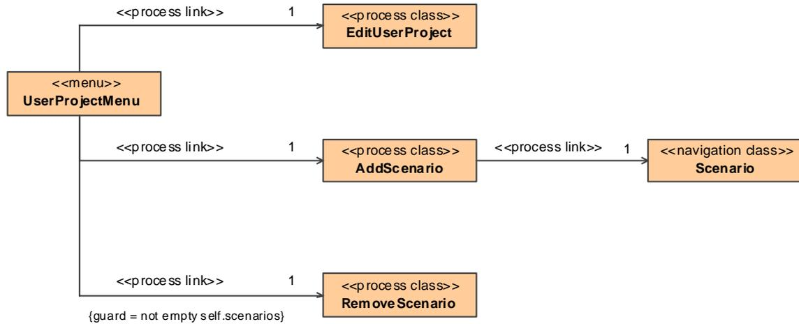
**Figure 113. Manually refined process classes and links for content class *UserProject***
