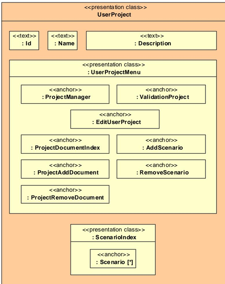
Figure 130. Automatically derived presentation classes for the navigation class *UserProject*, the menu *UserProjectMenu* and the index *ScenarioIndex*
