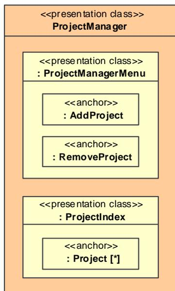
Figure 127. Automatically derived presentation classes for the navigation class *ProjectManager*, the menu *ProjectManagerMenu* and the index *ProjectIndex*
