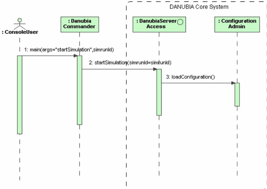
Figure 137. Offline starting of a simulation run
