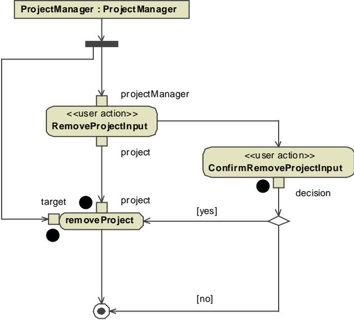
Figure 147. Token flow when executing process *RemoveProject* – step 5
