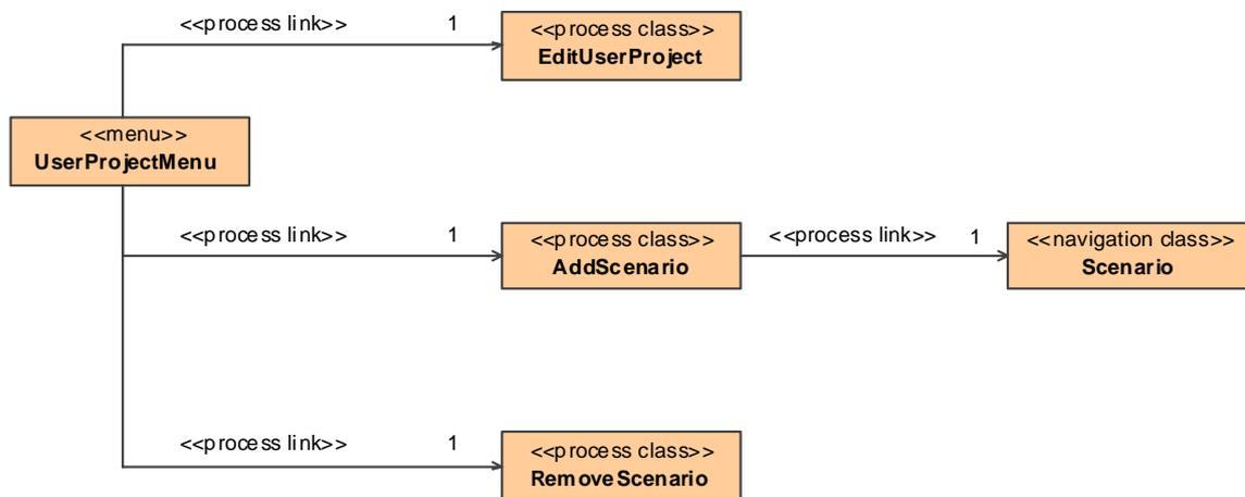
Figure 110. Automatically derived process classes and links for content class *UserProject*
