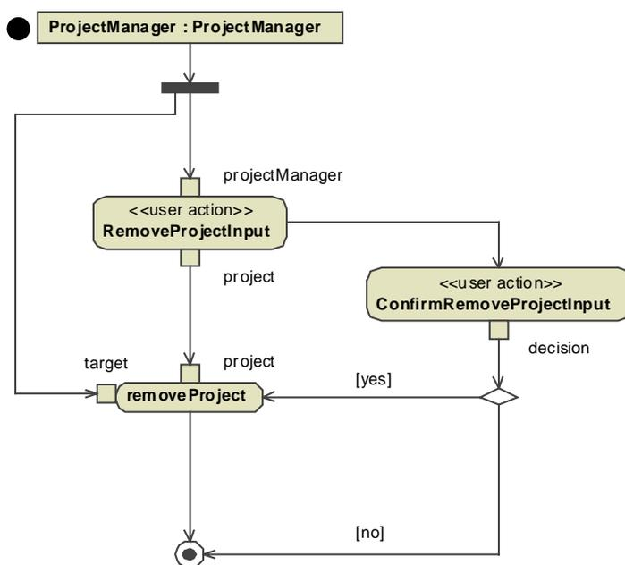
Figure 143. Token flow when executing process *RemoveProject* – step 1
