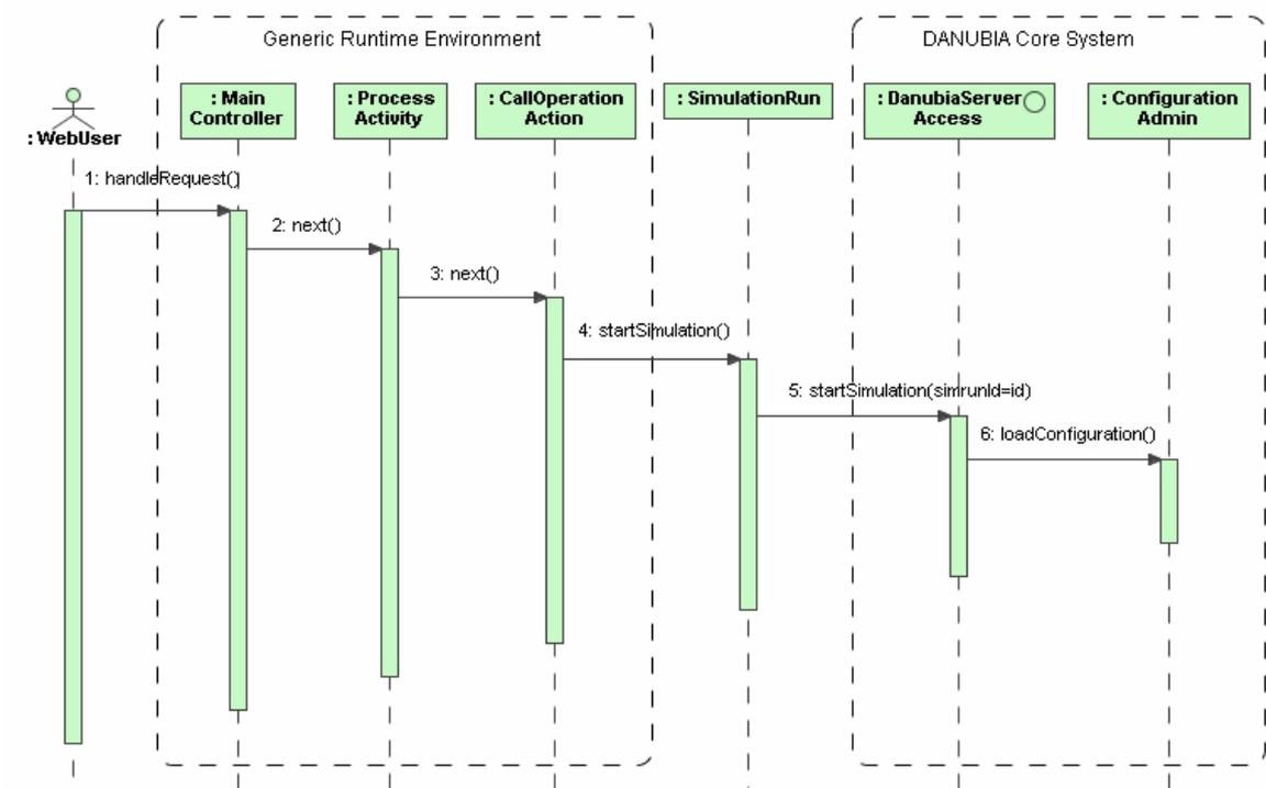
Figure 136. Online starting of a simulation run
