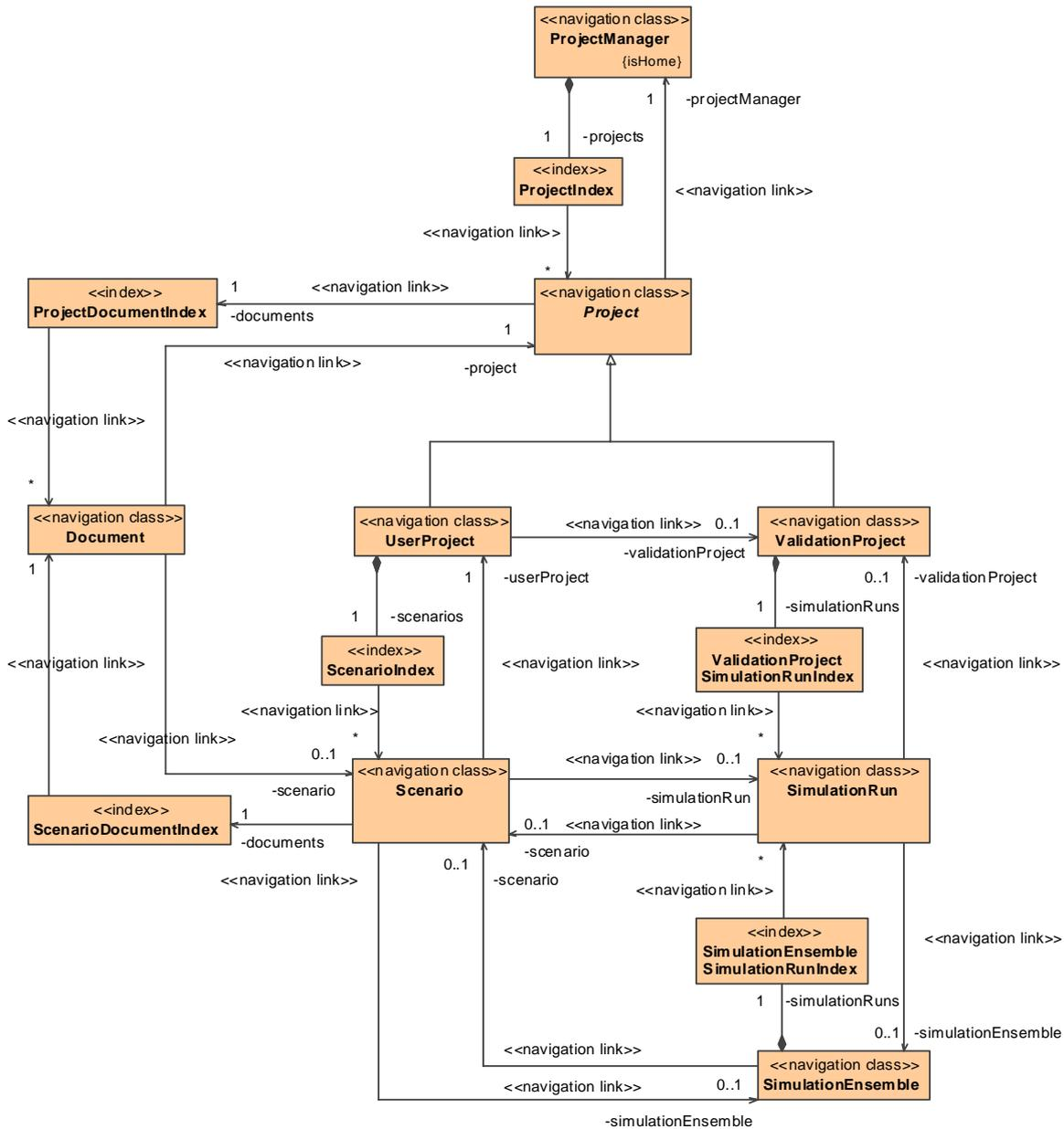
Figure 104. Navigation model after manual refining the automatically added indices
