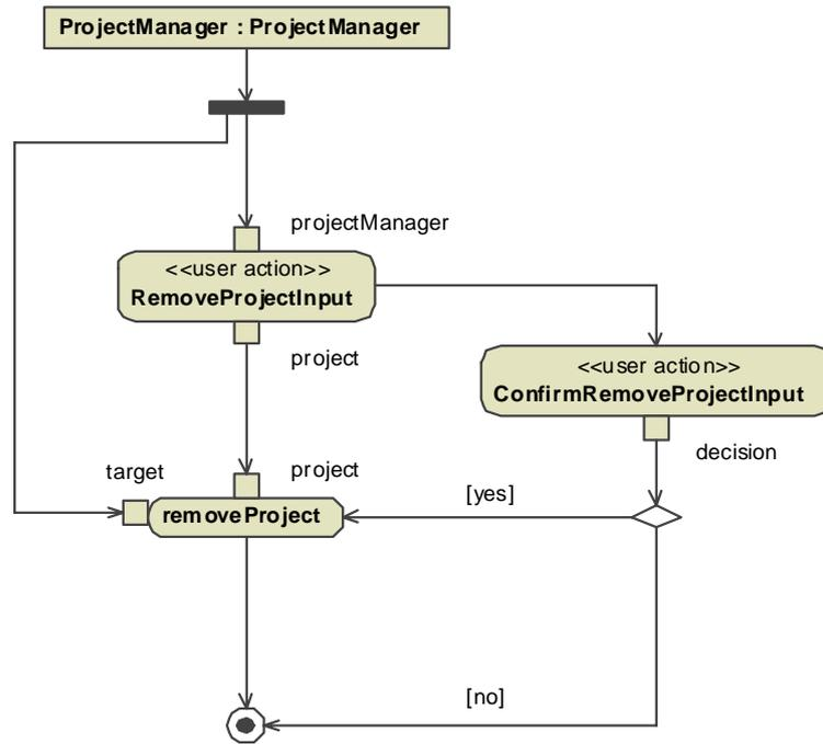
Figure 123. Manually refined process flow for process *RemoveProject*
