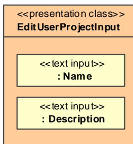
Figure 131. Automatically derived presentation class for the process class *EditUserProjectInput* of process *EditUserProject*
