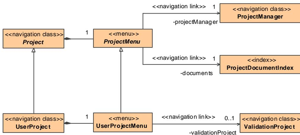
Figure 106. Navigation model with added menus derived by the transformation *AddMenus*
