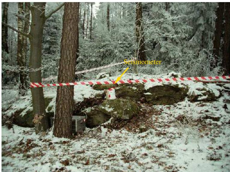
*Figure 3.3: Station S4 is located on outcropping large igneous rock boulders.*
