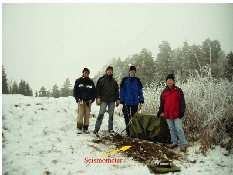
Figure 3.2: Station S1 located near a farm with the sensor was buried with a bottom depth about 50 cm.
