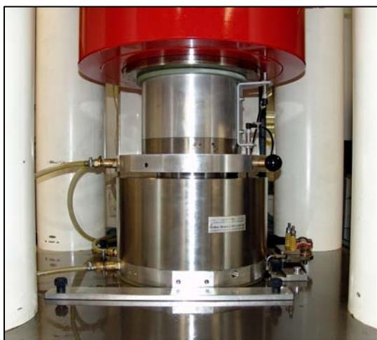
**Figure 2.2-23:** Loaded Walker-Module with fixed water cooling.
