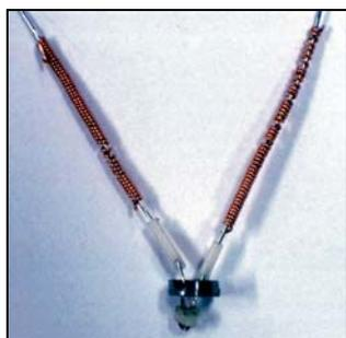
**Figure 2.2-31:** Axial thermocouple with copper coils, alumina sleeves and Mo ring [30].
