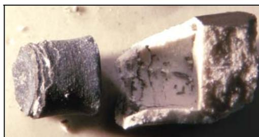
**Figure 2.2-36:** Separation of an intermetallic phase from a BN capsule [30].
