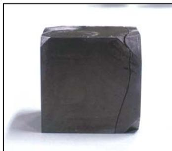
**Figure 2.2-38:** WC cube with crack [30].
