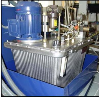
**Figure 2.2-9:** Main hydraulic unit and oil reservoir
