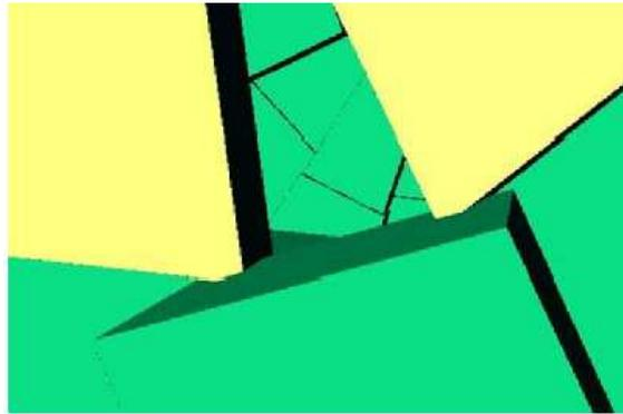
**Figure A.3:** Overlappings of the EIS1 chamber of the longbeam volumes of the chamber spacer with CSL1 chamber. This was due to the fact that CSL stations had no *coffin shape* at this stage of implementation.
