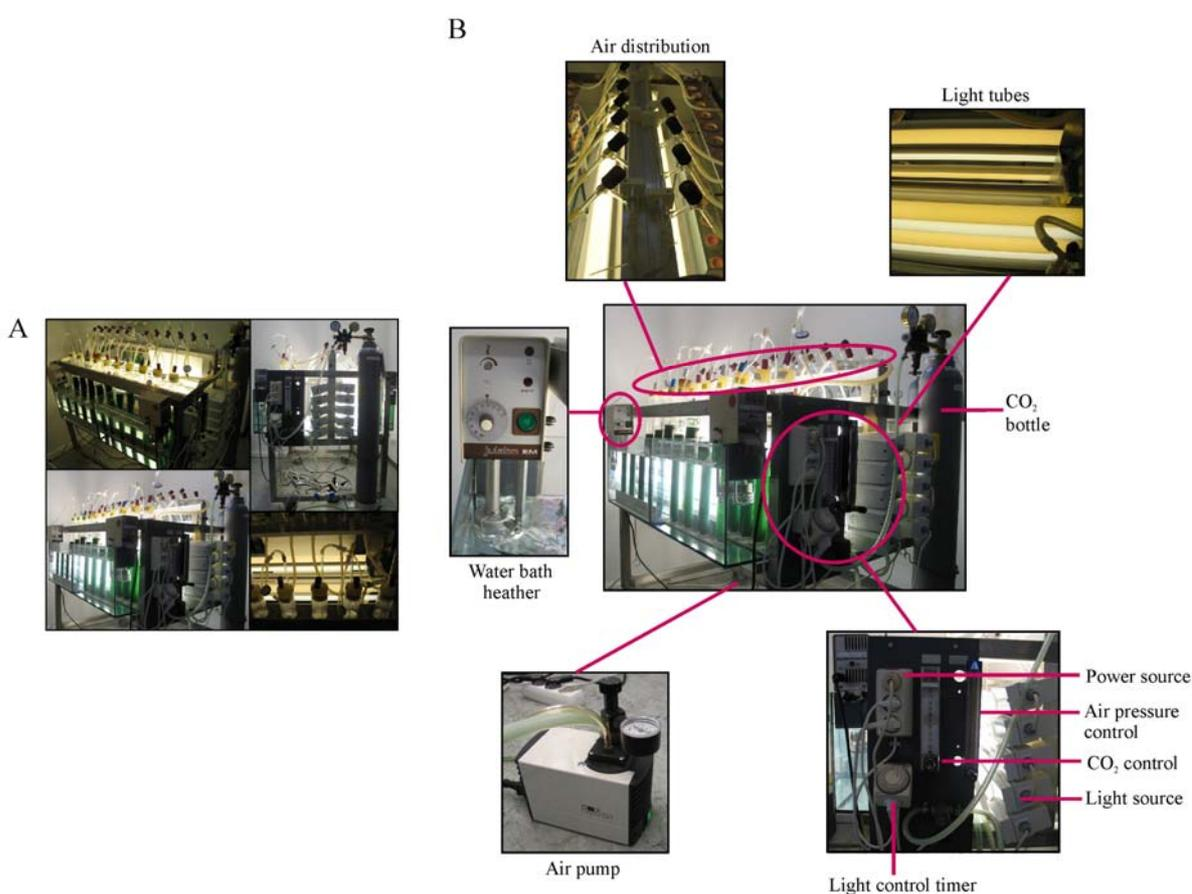
**Figure 5.** System used for the growth of air/CO<sub>2</sub> bubbled cultures of *Anabaena* sp. PCC 7120; (A) presents the complete system and (B) presents the more important parts separately.
