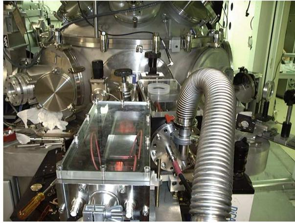
**Figure B.2:** Photograph of two Thomson parabola spectrometers (in the foreground) attached to the LULI 100TW target chamber.
