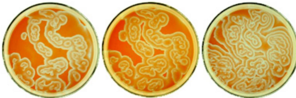
Figure 4.6: *The Belousov-Zhabotinsky reaction: In an unstirred mix of sodium bromate, ferroin, malonic acid and sulfuric acid in a petri-dish, changes of the concentrations of ferroin (red-orange) and ferrin (colorless-blue) ions are propagating in spiral-like waves.*
