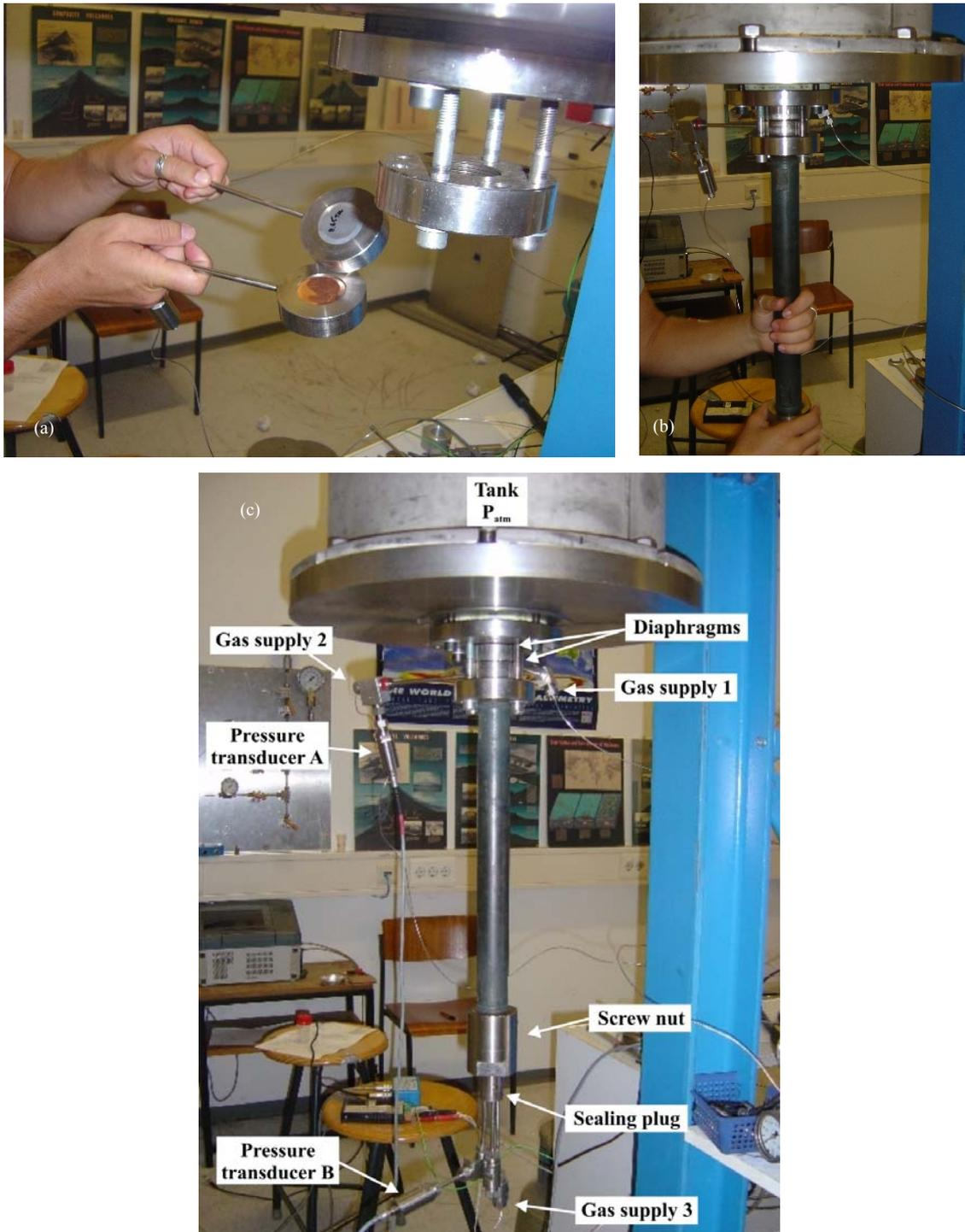
**Figure A3:** Copper or aluminium diaphragms are placed in the diaphragm holders (a). The autoclave is then attached to the tank and screwed down tightly against the diaphragms (b). Finally the gas supply system and the pressure transducers are attached (c).
