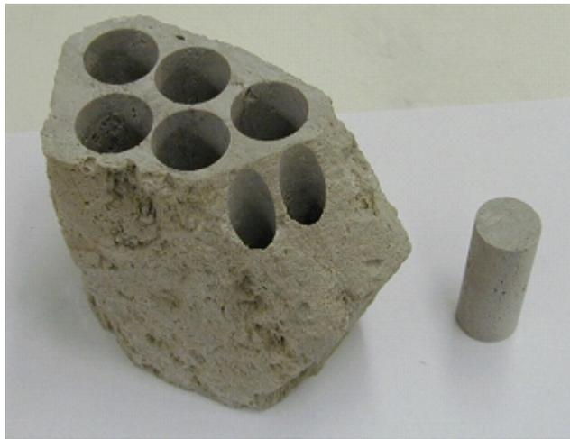
**Figure 2.30:** Pumice clast with a drilled sample cylinder. Height of the cylinder is 60 mm, the diameter is 25 mm.
