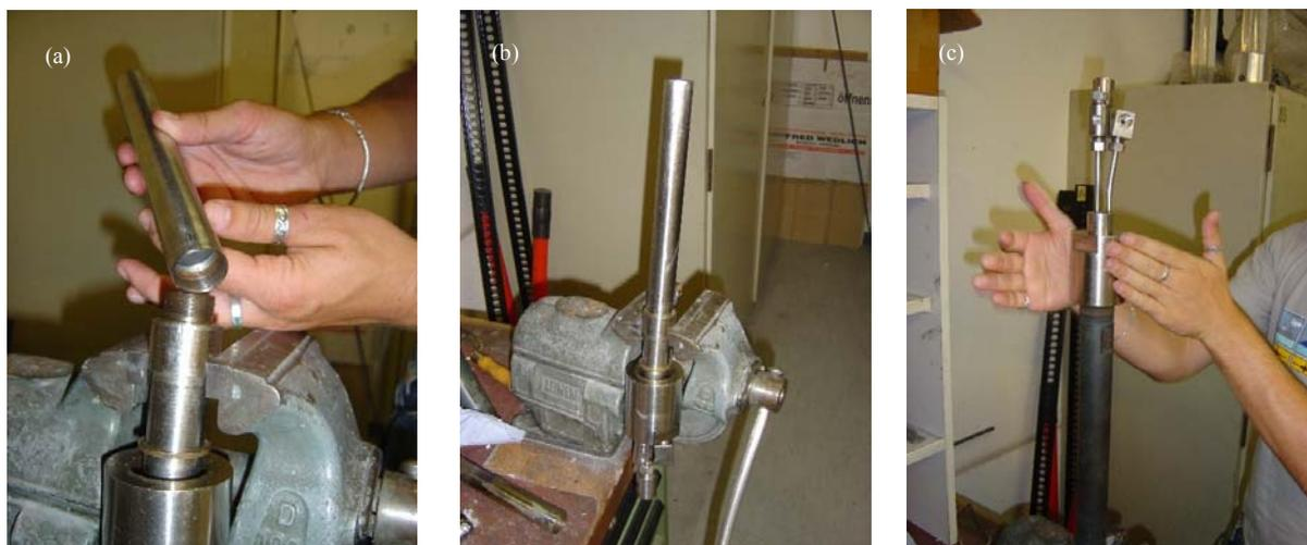
**Figure A2:** The steel tube is attached to the lower sealing plug (a) and screwed down tightly (b). Subsequently the sample tube is inserted into the autoclave, and the system is sealed with screw nut (c).
