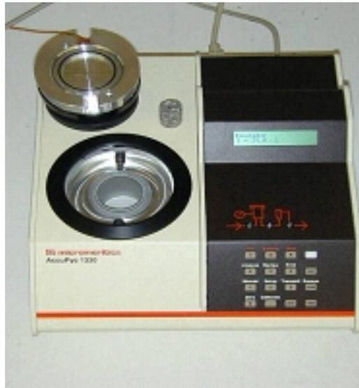
**Figure 2.31:** Density and porosity of the samples were determined in the laboratory using a helium pycnometer (Micromeritics AccuPyc 1330).
