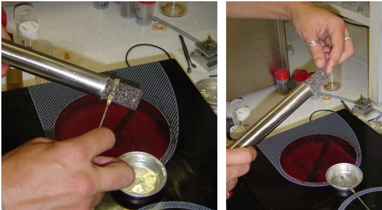
**Figure A1:** The sample cylinder is glued into the steel tube using Crystalbond™.
