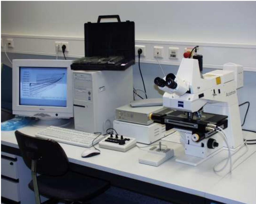
**Figure 5.6:** Automated scanning and particle counting station: The CR-39 detectors are placed under a computer controlled microscope. A CCD-camera relays the image to the computer where a special pattern recognition software searches for particle tracks. The tracks are counted and analyzed. From the stored data the complete image on the CR-39 can be reconstructed, displayed and further processed.
