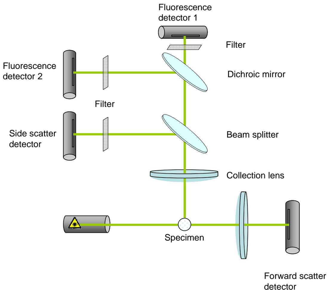
**Figure 8: Basic optics of a flow cytometer.**
