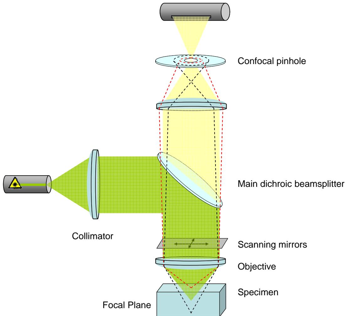
**Figure 9: Principle of confocal laser scanning microscopy**
