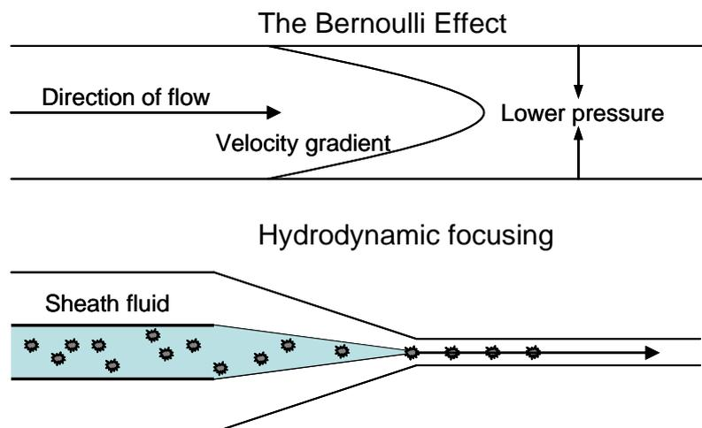
Figure 7: Fluidics and hydrodynamic focusing.
