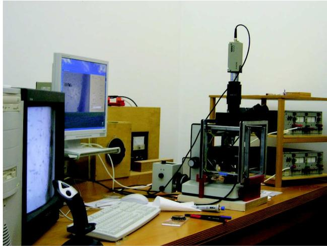
Figure 3.3: The Bacteriodrome used to study the swimming behavior of MTB and to concentrate cells. The light microscope is surrounded by two pairs of coils which allow for a control of the ambient field both in intensity and horizontal direction.
