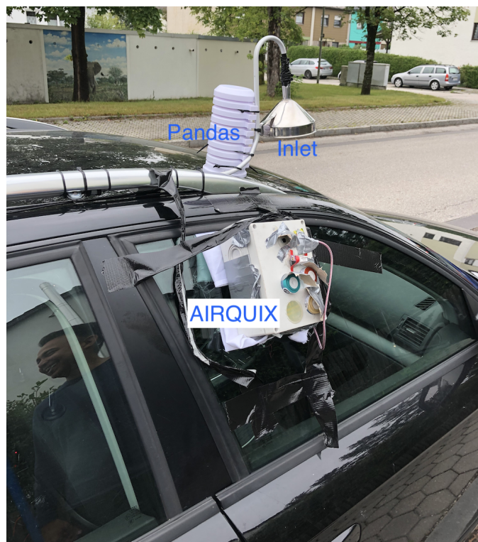
Figure 6.8: Inlet setup of Vehicle 1 used in the AIRIDE campaign.
