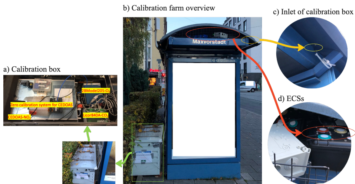
Figure 4.1: Reference air quality monitoring station as calibration station with ECSs and CE-DOAS instrument
