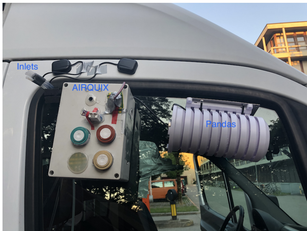
Figure 6.9: Inlet setup of Vehicle 2 used in the AIRIDE campaign.
