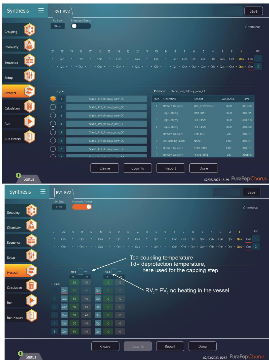
Figure S3. Views of the protocol sub-window where the protocol for a given cycle is selected and the target temperatures for coupling and capping are saved.
