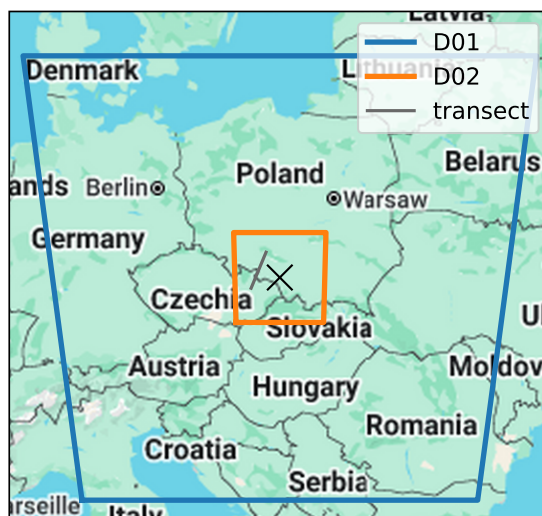
Figure 4.5: Nested model domains used in the WRF-Chem simulation. Both domains are square and centred over the USCB. The outer domain (D01) spans 1400 km with a horizontal resolution of 5 km, while the inner domain (D02) covers 280 km at 1 km resolution. The virtual transect marked in D02 corresponds to the vertical cross-section shown in Fig. 4.6b-c.
