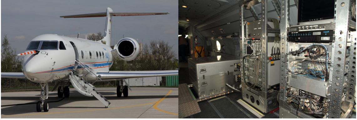
Figure 2.1: Left: the German research aircraft HALO before take-off. Right: inside High Altitude and Long Range Research Aircraft (HALO)'s cabin, showing the full CHARM-F system. From left to right: lasers and receivers; laser cooling and controlling; PCs for laser operation, wavelength stabilisation and data acquisition. Both photos taken by A. Fix.
