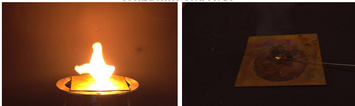
Figure S24. Reaction of [\text{Cu}(\text{2-AET})_2(\text{PA})_2] during hot plate (left) and hot needle test (right).
