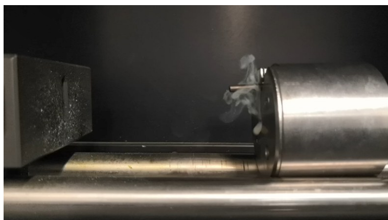
Figure S74. Decomposition of [\text{Cu}(\text{PA})_2(1\text{-TAN})_2] during laser irradiation (10 A, 30 ms, 4 V).
