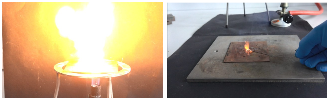
Figure S53. Reaction of [\text{Cu}(\text{1-AT})_2(\text{HTNO})_2] during hot plate (left) and hot needle test (right).
