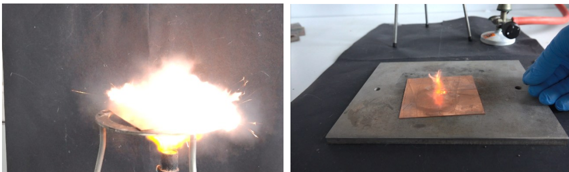
Figure S65. Detonation of PbTNO during hot plate (left) and hot needle test (right).
