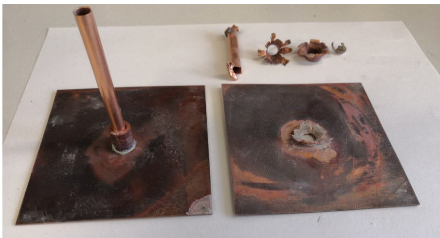
Figure 11. PETN initiation setup. Left: negative attempt with no damage to shell or plate, right: positive initiation by 10 .
