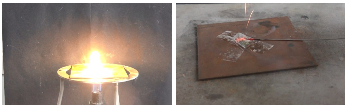
Figure S18. Hot plate (left) and hot needle (right) test of compound 8 .
