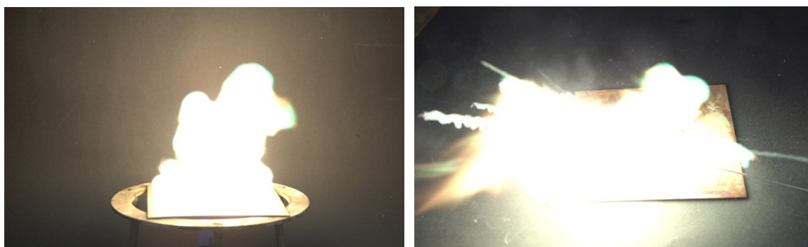
Figure S22. Reaction of [\text{Cu}(2\text{-AET})_4(\text{H}_2\text{TNPG})_2] during hot plate (left) and hot needle test (right).
