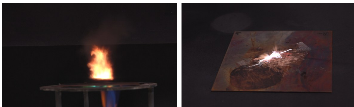
Figure S29. Detonation of [\text{Cu}_2(2\text{-AET})(\text{N}_3)_4] during hot plate (left) and hot needle test (right).
