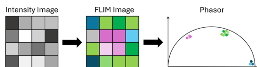
Figure 2: Schematic drawing showing the relationship between the intensity grayscale image (left), the FLIM image (center) and the phasor plot (right). With a lifetime capable microscope, in addition to the intensity image, the lifetime image can be recorded, where every pixel has an average lifetime value. From these values a phasor can be created. Pixels with similar long lifetimes (pink), similar intermediate lifetimes (green), and similar short lifetimes (blue) will form clusters on the phasor plot.
