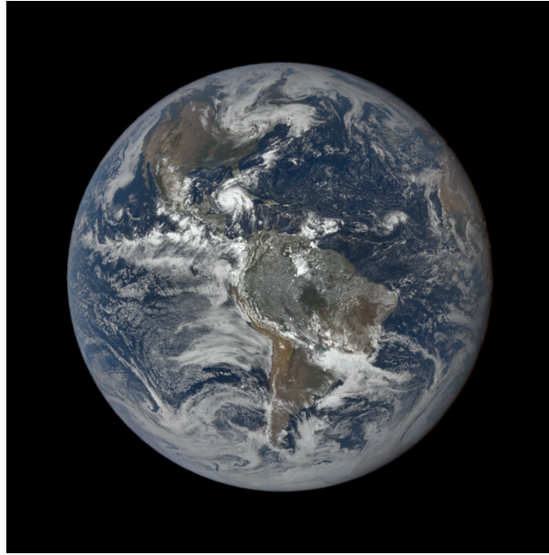
Figure 1.2: DSCOVR/EPIC natural color image of Earth on September 26 th 2022. The natural color images are produced using the bands of the EPIC instrument within the human visual range and adjusted to simulate what a conventional camera would reproduce. Image credits: NASA/DSCOVR.
