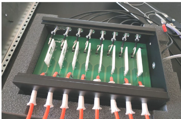
Figure 3.14: Voltage divider installed at the FRS-IC setup. It is made of an 8-fold resistive voltage divider, which enables a continuous monitoring of the voltages at the TOF analyzer electrodes.
