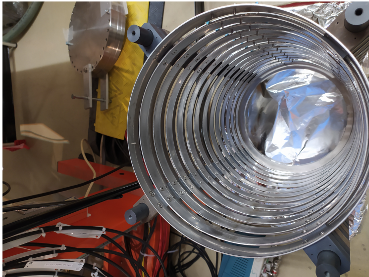
Figure 3.4: The "short" DC cage shown in this picture is a cylindrical electrode structure consisting of 27 rings with a length of 48.2 cm and a diameter of 26.7 cm.
