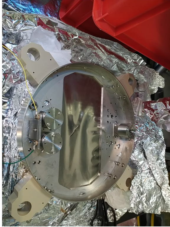
Figure 3.5: The first ring of the DC cage is a metallic place installed at the entrance side on top of the DC cage is made up of 3 sections to place the source holders and in the central part a window made up of a degrader (a Ti foil of 30\text{ }\mu\text{m} thickness). The source holders on the left have ^{228}\text{Th} and ^{148}\text{Gd} radioactive sources installed, in the source holder on the right ^{252}\text{Cf} source is installed.
