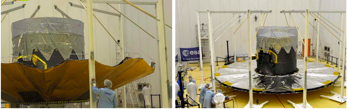
Figure 1.8: Gaia flight model undergoing a deployment test of its foldable sunshield while in Kourou, French Guiana, awaiting launch in December 2013. The engineers in the foreground provide a sense of the satellite’s size. Image credit: ESA–M. Pedoussaut, 2013.
