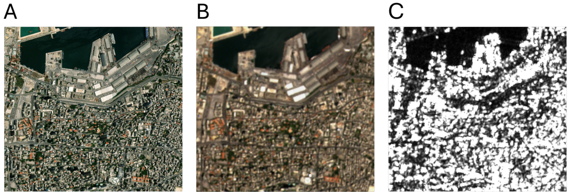
Fig. 1: Comparison of satellite images of the Beirut harbor, July 2020. (A) is a proprietary high-resolution (30cm) optical image from Maxar WorldView-3. Due to the harbor explosion, the image was made freely available by Maxar [Maxar Technologies, 2024]. (B) is a publicly available optical image with medium-resolution (10m) from Sentinel-2A, using bands 4, 3 and 2. (C) is a publicly available multi-looked SAR image with medium-resolution (20m after processing; see Methods for details) from Sentinel-1. It is one of the images used in our detection. For visualization of the two-dimensional image of complex samples with a real and imaginary part, we use a \gamma_0 greyscale visualization of the VV polarization.
