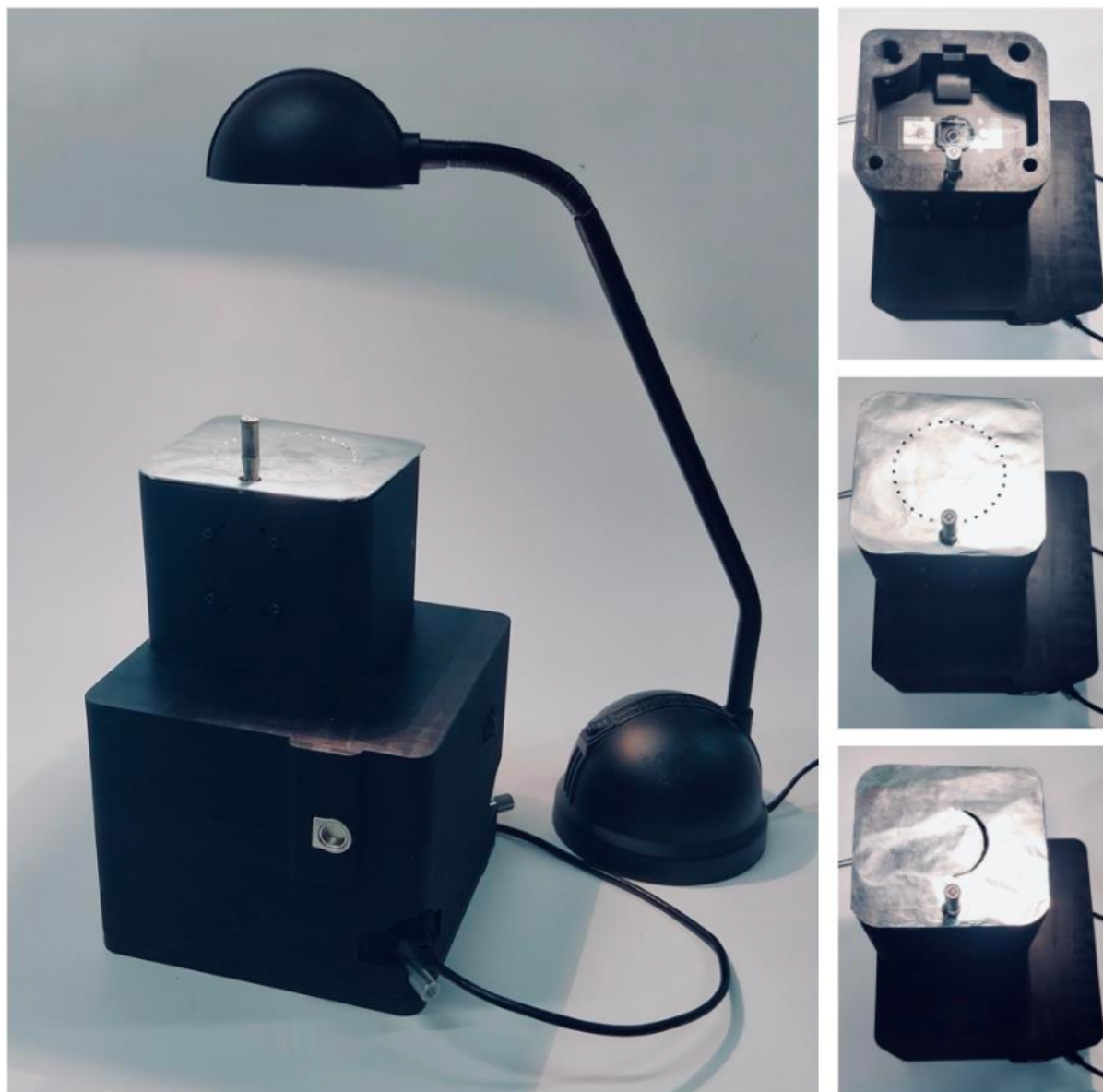
Figure 3.33: Transmission light microscopy using Brick-MIC. The left panel shows the Brick-MIC video modality with an LED desktop lamp used as light source, which was positioned right on top of the sample holder. The sample holder is covered with aluminum foil with a punctured circular pattern for darkfield imaging (middle right panel). The upper right panel shows an uncovered sample holder used for bright field imaging. The lower right panel shows the aluminum covering used for oblique illumination, where the foil has a punctured crescent moon shape.
