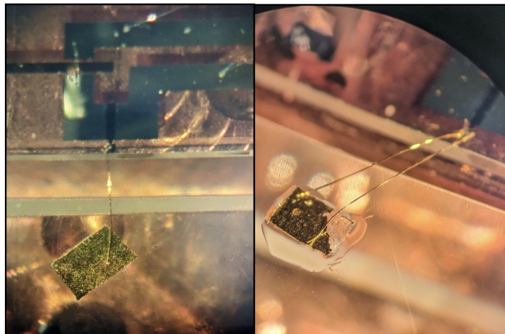
Figure 7.2: Close-up views of the Au-film ( 8\text{ }\mu\text{m} thick) glued onto an NaI crystal. The increased thickness improves handling and reproducibility.
