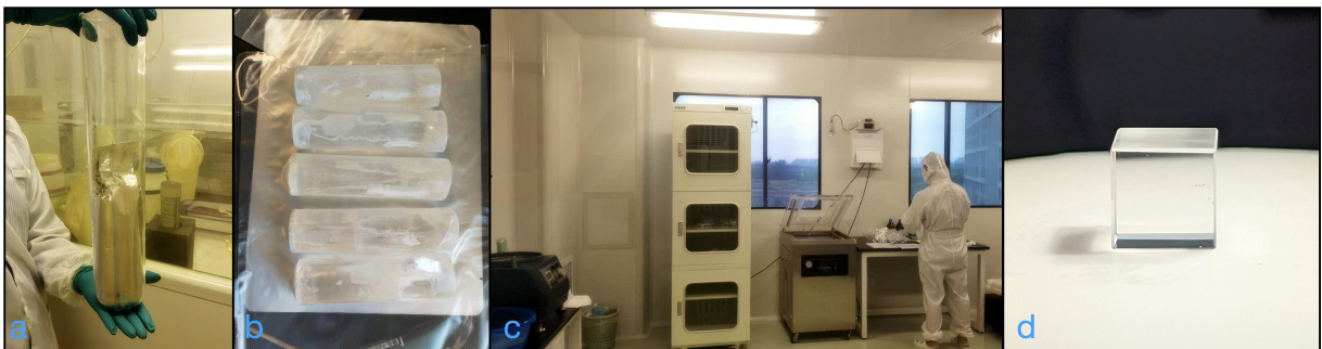
Figure 3.4: Crystal production process at SICCAS: From left to right: a) A quartz ( \text{SiO}_2 ) crucible lined with a Pt foil is used for crystal growth; b) NaI ingots obtained after the growth process; c) Dry clean room for mechanical processing and polishing of the crystals; d) A polished (21 \times 21 \times 21) \text{ mm}^3 radio-pure crystal in a nitrogen-flushed, moisture controlled glove box prepared for R&D measurements.
