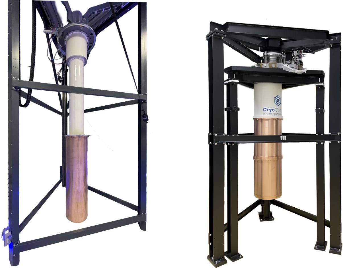
Figure 4.11: The COSINUS dry dilution refrigerators (images are not to scale). Left: The dry dilution refrigerator (nicknamed Calippo) installed at LNGS, prior to being lowered into the drywell for it's first cooldown; Right: The dry dilution refrigerator (nicknamed Giovanni Giorgio) installed at MPP, ready for it's first cooldown at the Garching campus.
