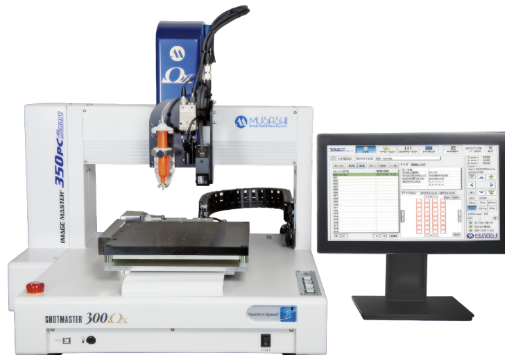
Figure 7.8: The Musashi 350PC Smart automated dispensing system used for precise pneumatic deposition of Epo-Tek 301-2. It offers fine control over glue spot diameter and thickness by adjusting air pressure, dispensing time, and nozzle size. Different glue-spot patterns can be programmed via the built-in Mu-CAD software for various crystal sizes.
