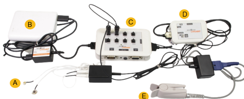
Figure 5.5: The medical-grade system used as gold standards for evaluating SensCon-based EDA and PPG measurements. The EDA electrodes (A) and PPG finger clip sensor (E) are connected to the AUX ports of the Sensor & Trigger extension (STE) (C). For signal amplification and streaming to the acquisition PC, we use a LiveAmp amplifier (D) and a power bank for energy supply to the STE (B). All components were placed inside a pouch and comfortably worn by participants across the experimental sessions
