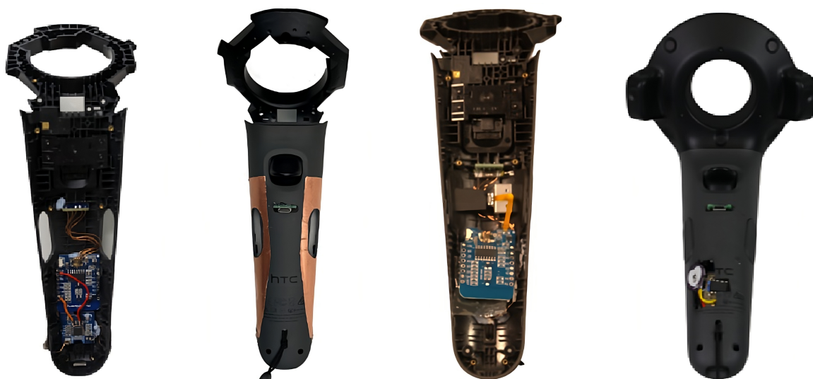
Figure 5.3: EDA and PPG sensors integrated into VR controllers. In the first picture, EDA sensor is integrated into a controller. In the second figure, two copper stripes measure the EDA when a user picks up the controller. In the third figure, PPG sensor integrated inside the controller. In the fourth figure, the PPG sensor measures the user's HR by implicitly pressing the palm against the sensor.
