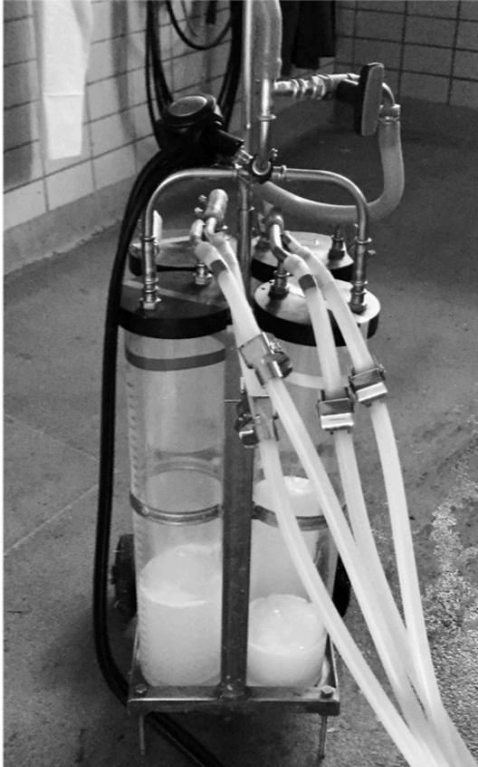
**Fig. 7** Quarter milking system. Photo of the quarter milking system, which was used every 12 h during the challenge experiment to milk the cows to assess the milk yield and representative full milk samples at the quarter level
