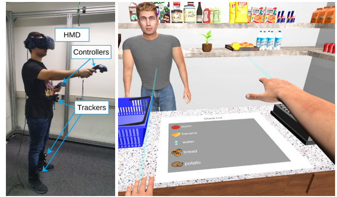
Fig. 6. Embodiment method. HTC VIVE Pro Eye and HTC VIVE trackers that allow for the embodiment of the user in the simulation by using inverse kinematics and body pose solving.
