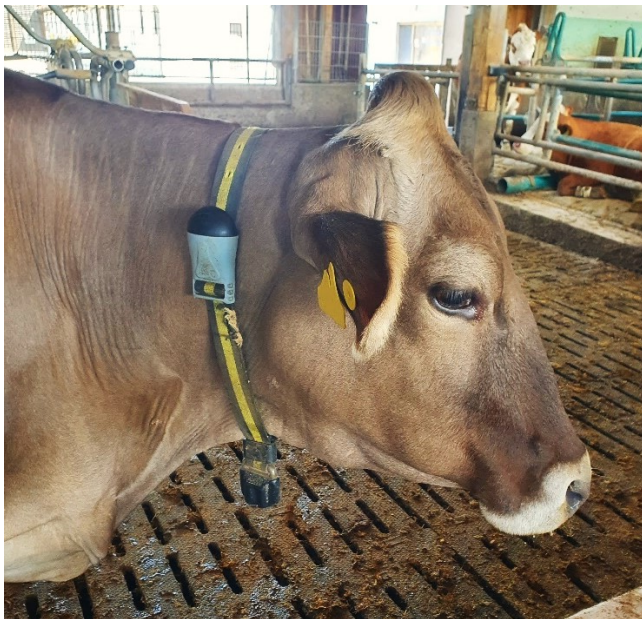
Figure 22: SCR HR-LDn neck tag
