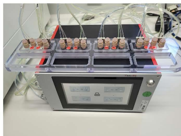
Fig. 2. The HUMIMIC starter platform (TissUse, Berlin, Germany) with the respective HUMIMIC Chip2 experimental setup for the determination of VX toxicokinetics.
