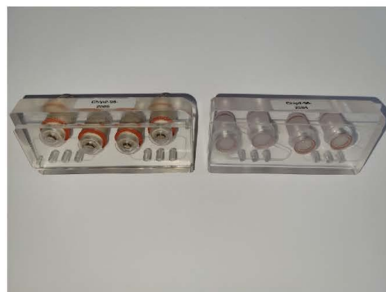
Fig. 1. The HUMIMIC Chip2 96-well co-culture model from TissUse (Berlin, Germany). On the left side, the polydimethylsiloxane-based (PDMS) chips and on the right side, the cyclic olefin copolymers-based (CoC) chips are illustrated.
