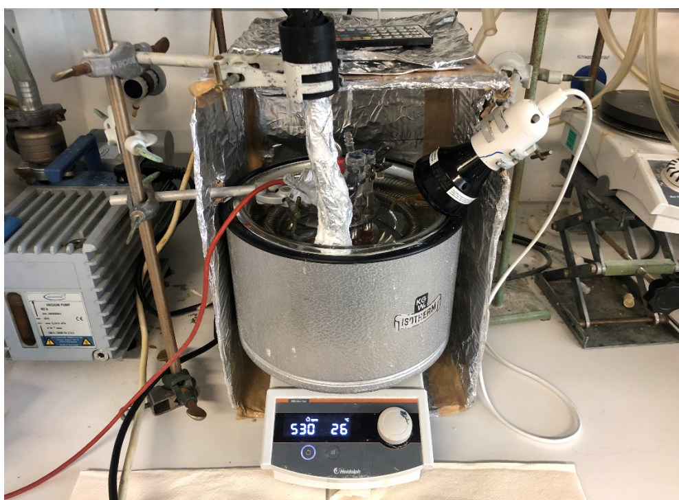
Figure 10: Photochemical Setup for low-temperature Reactions
