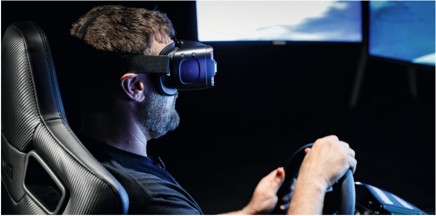
Figure 2.7: In this image, the professional drifter Vaughn Gittin Jr. drives an AV remotely using a steering wheel and pedals as input devices and an Head Mounted Display as output devices. An image from the 2019 Samsung Press Kit.
