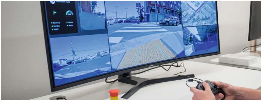
Figure 2.3: In this image, a Phantom Auto remote operator controls an autonomous mobile delivery robot via a dual joystick controller that asked for support. An image from the 2020 Phantom Auto Press Kit.
