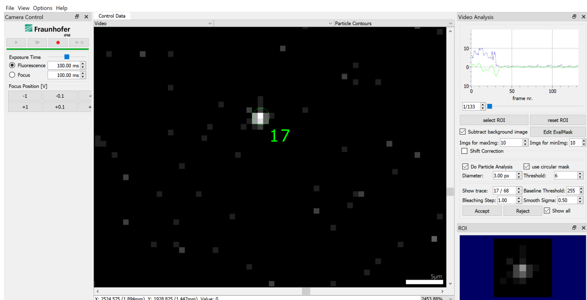
Figure D. A snapshot of the software showing a detected single molecule and the time transient on the top right showing a single bleaching step.
