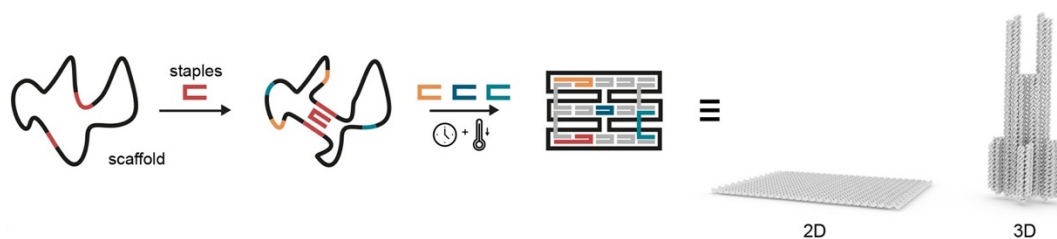
Figure 14. Schematic for DNA Origami folding technique to create two- or three-dimensional nanostructures. Copyright 2021 45 . Published by American Chemical Society, licensed under CC-BY-NC-ND 4.0
