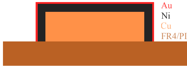
Figure 8.5: Sketch (not to scale) of a strip on the insulator made of either FR4 or PI. The strip consists of copper coated with nickel and a layer of gold. In the simulation, the ENIG coverage is approximated by neglecting the side areas and only covering the top surface area. Design information extracted from [Multi Circuit Boards, 2024a].
