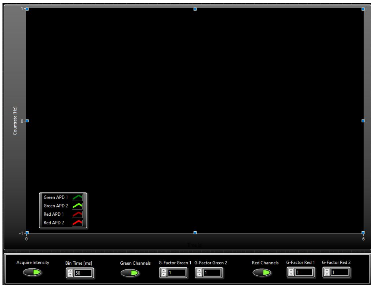
Figure 4.4: GUI of the Acquire Intensity subVI. In this interface, the count rates of both detector pairs are displayed. The user can define the binning time parameter and activate the channels.
