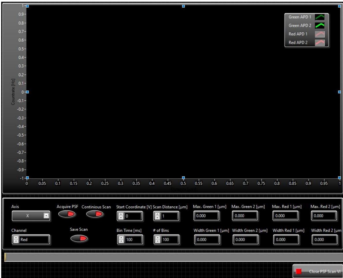
Figure 4.5: GUI of the PSF scan subVI. In this subroutine, detection channel and coordinate axis on which the PSF scan is performed can be chosen. Furthermore, the number of data points per scan, binning time [ms] and scan range [ \mu\text{m} ] can be defined. The scan is displayed on screen in real time.
