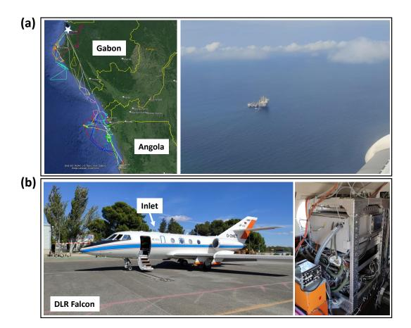
Figure 5.7: (a) Flight tracks of the 15 MTGA flights off the coasts of Gabon and Angola. A photograph of an oil platform as seen from the research aircraft is shown on the right. (b) Photograph of the DLR Falcon (Dassault Falcon 20 E-5) research aircraft on the left and the DLR-QCLS mounted inside the cabin on the right side.
