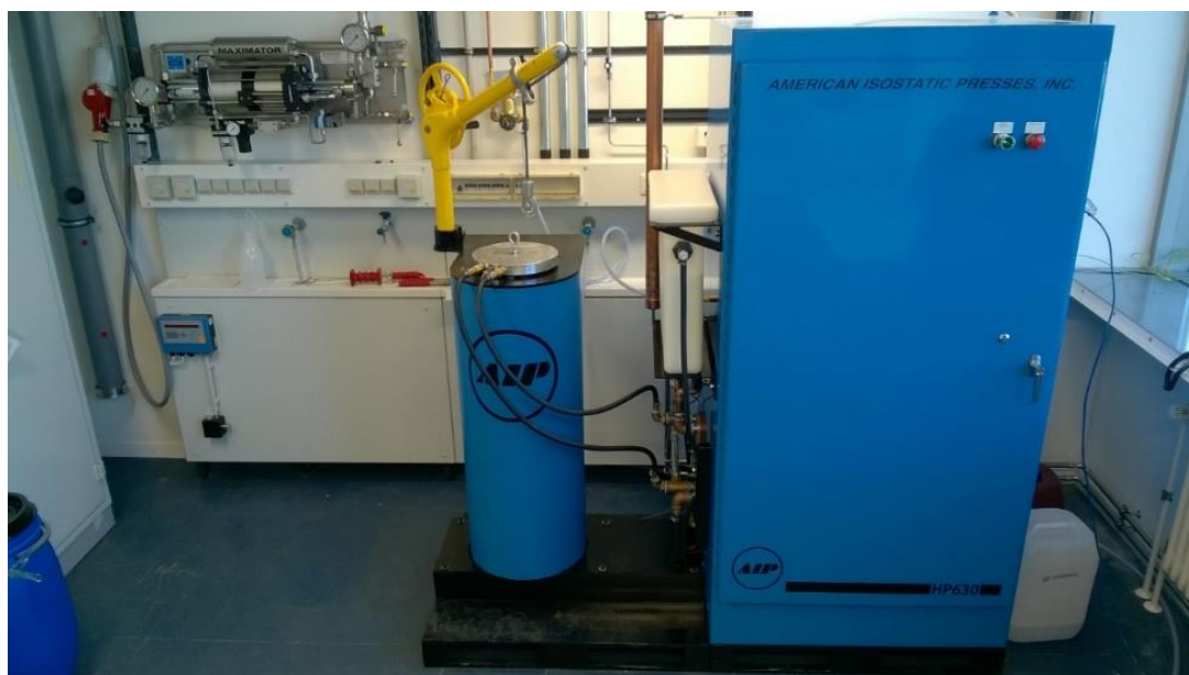
Figure 1.7. HIP (AIP6-30H, American Isostatic Presses Inc., Columbus, USA). Left top: Pressure booster (Maximator, DLE-5-30-2); center: Pressure vessel with crane for lifting the threaded lid and coolant lines; right: control cabinet (control electronics, valves, pumps and main compressor).
