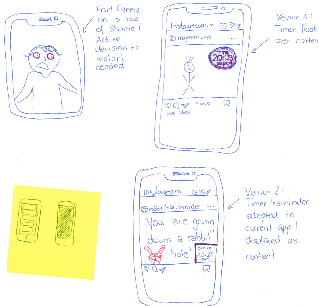
Figure 3.6 : Four resulting sketches from our experts' focus group on the question of communicating MPRH to the user. From left to right : (1) A user terrified of their image in the black mirror, after being in a MPRH. (2) Floating timer. (3) Quick shutting down of the screen once MPRH was detected. (4) Timer blended in content, as Instagram post.
