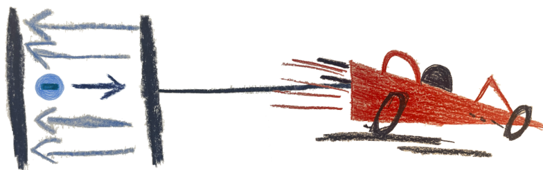
Figure I.1: A simple particle accelerator: A capacitor pulled by a race car. Electrons acquire kinetic energy by falling along the electric field lines in a capacitor. Their final energy is proportional to the field amplitude and the spacing of the plates. If the capacitor co-moves at the velocity of the electrons, the possible energy gain is limited only by the energy the car supplies to the system. Drawing inspired by [1, 2].
