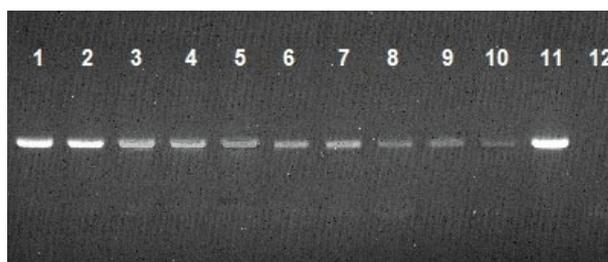
FIG. 1: Comparison of two DNA extraction kits (Analytik Jena, AJ; Zymo Research, ZR) on all sample materials with 100bp DNA ladder. 1: AJ gauze, 2: AJ swab, 3: AJ filter paper, 4: AJ prefilter, 5: AJ nestlet, 6: ZR gauze, 7: ZR swab, 8: ZR filter paper, 9: ZR prefilter, 10: ZR nestlet, 11: positive control, 12: negative control.
