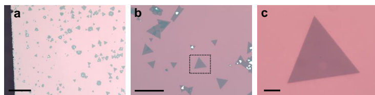
Figure 4.13: Growth result of \text{WSe}_2 . a , Distribution of different shapes and sizes, well-separated. b , Well-separated triangular crystals of high quality. c , Dotted square in b . Scale bars are (left to right): 300, 100, and 10 \mu\text{m} .
