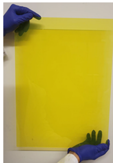
Figure 4.10: Nanocomposite of CsPbBr 3 perovskite nanocrystals in a polymer under ambient light. Figure from Erroi, Frank et al. [28], reprinted under CC BY 4.0.
