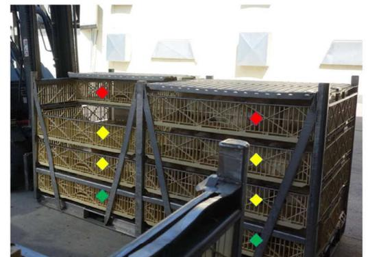
Figure 2. Metal container of the type GP live bird container supply system from the company Marel (Austurhraun 9, Gardabaer, IS-210 Iceland). The container consisted of a metal frame with a total of 8 crates, divided into 2 sides (left and right) with 1 low (green), 2 middle (yellow), and 1 high crate (red) on each side; each crate is opened and closed manually during loading.
