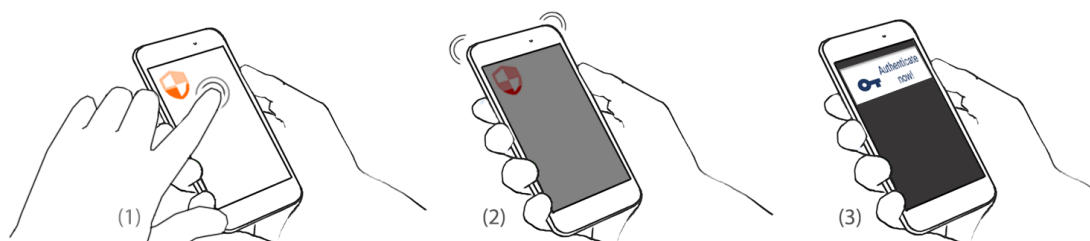
Figure 8.1: We propose to use indicators to communicate both the current device confidence level ( DCL ) and the need for re-authentication for continuous implicit authentication systems on mobile devices: 1) a long term indicator illustrates the current DCL and its development over time via a taskbar icon, and 2) a short term indicator announces an upcoming re-authentication via darkening the screen. Our system also allows for 3) voluntary re-authentication to avoid system-side locking of the device.
