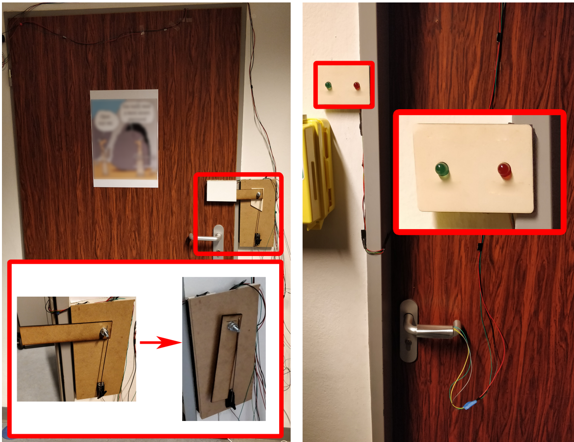
Figure 4.4: Left: The back view of the door. The mechanical door lock was controlled over a wireless network. Right: The front view of the door. Additional feedback regarding the success of an authentication attempt was provided by colored lights at the front side. The green LED on the left indicates success, and the red LED on the right failure.
