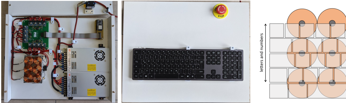
(a) The matrix of electromagnets is on the left and the power supply units are on the right side. The microcontroller is situated behind the power supply units. (b) Top view of our finished prototype. The keyboard is fixed with 3D-printed clamps and an emergency button is placed in the right corner. (c) Dimensions and placement of the electromagnets under the keyboard.
