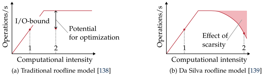
Figure 5.2: Comparison of the traditional roofline model and the model proposed by Da Silva with resource congestion
