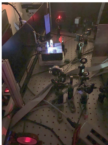
Figure S20: TA setup. The 365 nm LED illuminating constantly from the side is seen as a bright white-blue light.
