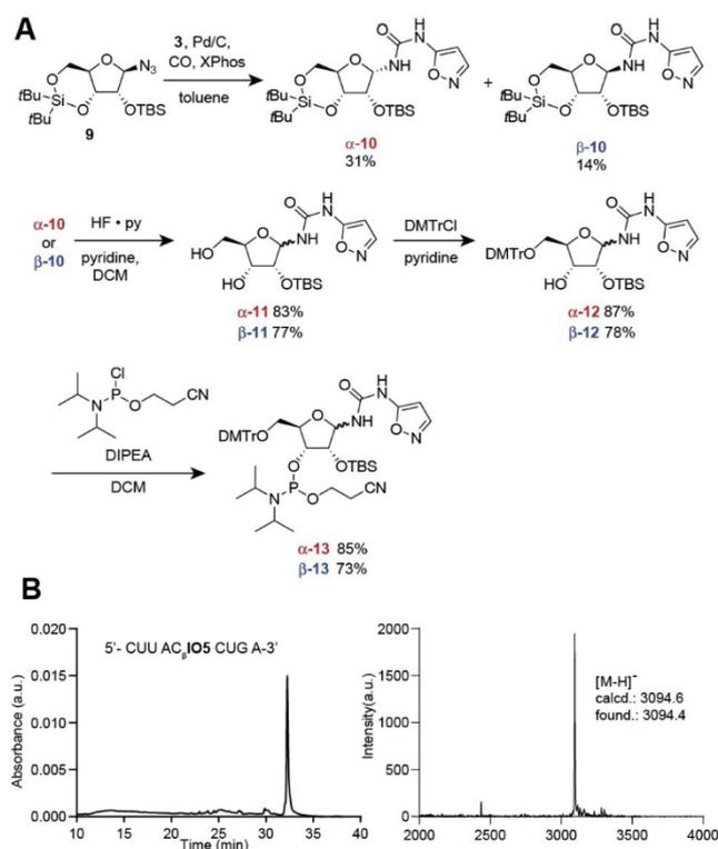
**Scheme 1.** A) Synthesis of the IO5 phosphoramidite and conditions B) HPLC-chromatogram and MALDI-TOF mass spectra of an oligonucleotide synthesized with the IO5 phosphoramidite  $\beta$ -**13** shown as an example.
