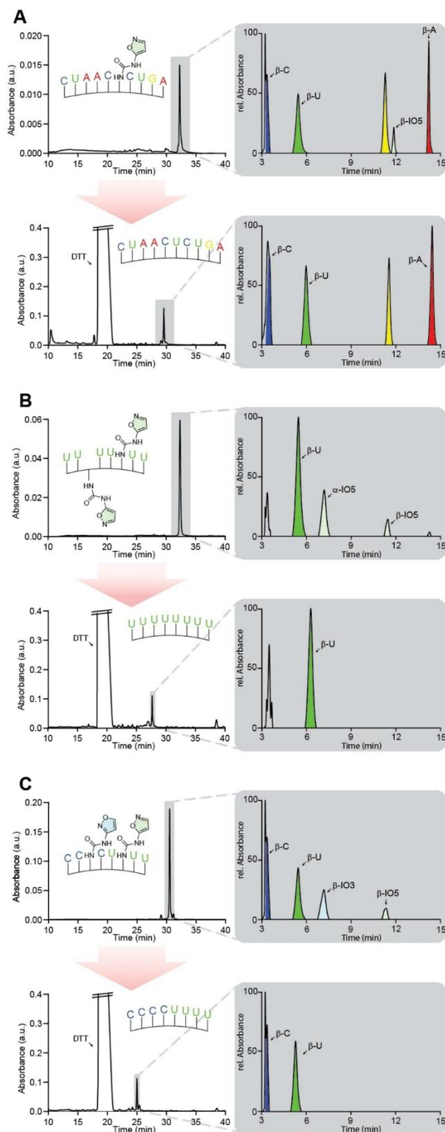
**Figure 3.** HPLC, MALDI, HPLC-MS (at 243 nm; grey brackets) analyses of the IO5 containing Strands before the reaction with DTT,  $\text{Fe}^{2+}$  (top) and after N–O cleavage and cyclization reaction (bottom). A) 5'-CUAAC- $\beta$ IO5-CUGA-3' B) 5'-UU- $\alpha$ IO5-UU- $\beta$ IO5-GA-3' C) 5'-CC- $\beta$ IO3-CU- $\beta$ IO5-UU-3'. A = adenosine, C = cytidine, G = guanosine, IO3 = 3-aminoisoxazole, IO5 = 5-aminoisoxazole, U = uridine.
