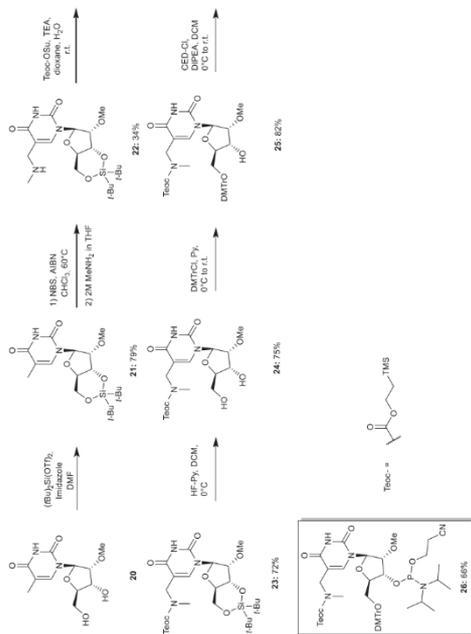
**Scheme S7.** Synthesis of nucleobase-modified 5-methyluridine 2'-methoxy phosphoramidite.
