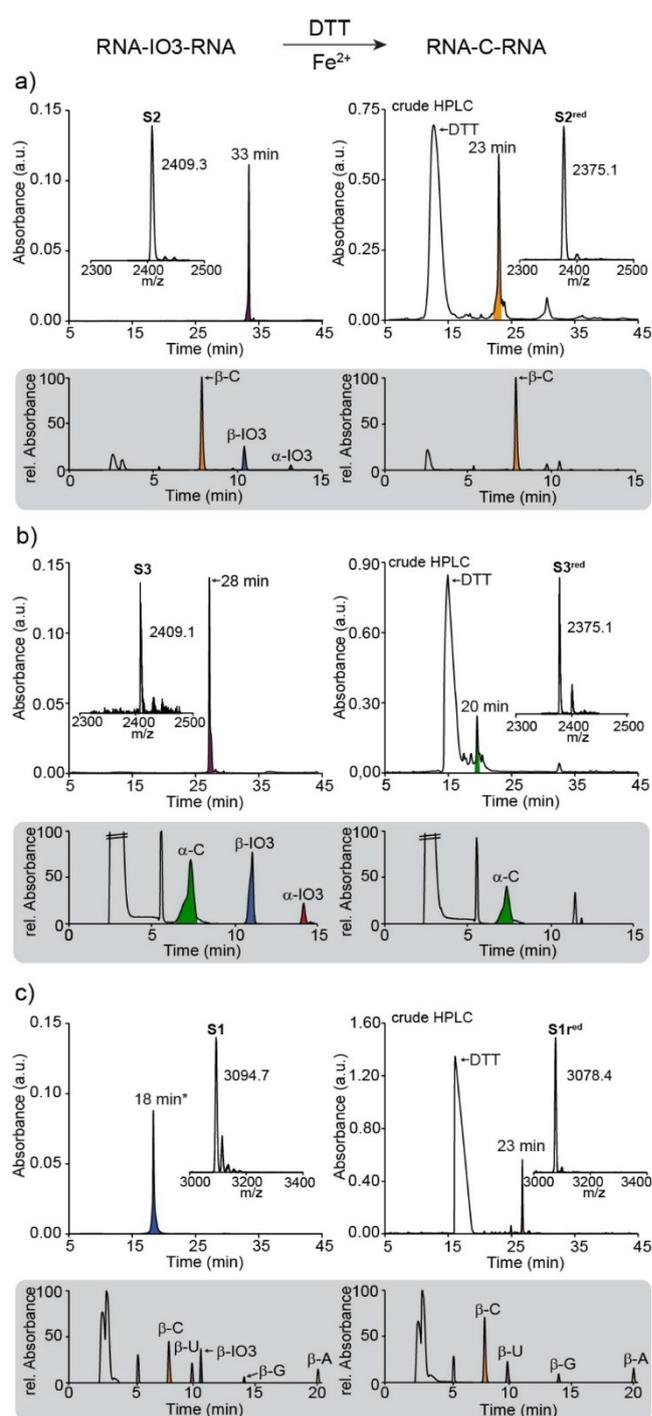
**Figure 2.** Reaction of the IO3 containing strands with DTT and Fe<sup>2+</sup> and HPLC, MALDI, HPLC-MS (at 223 nm; gray brackets) analyses of the N–O cleavage and cyclization reaction (left: starting material; right: product). a) Result of the  $\beta$ -homo-C strand **S2**; b) the  $\alpha$ -homo-C strand **S3**; c) the strand **S1**. A = adenosine, C = cytidine, G = guanosine, IO3 = 3-aminoisoxazole, U = uridine. \*HPLC gradient: 0–40% buffer B.
