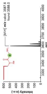
Figure S56. MALDI-TOF mass spectrum (negative mode) of the isolated ON5a (gmm<sup>1</sup>U).
