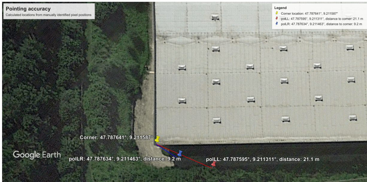
Figure 3.13: Google Earth image showing the same ground target as in Figure 3.12 and the corresponding offsets to the calculated positions from manually identifying the corner pixel in images of the poLLR (blue) and poLL (red) cameras.
