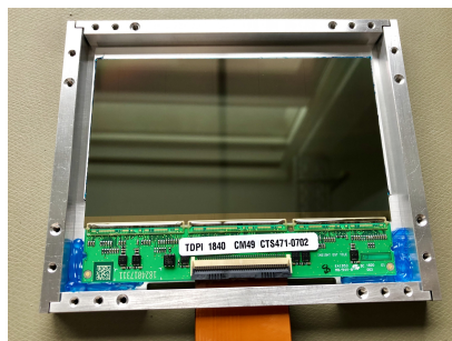
Figure 4.1: The CM49 sensor surface and the PCB containing the Analog-to-Digital Converter (ADC) units (from Englbrecht, 2022).
