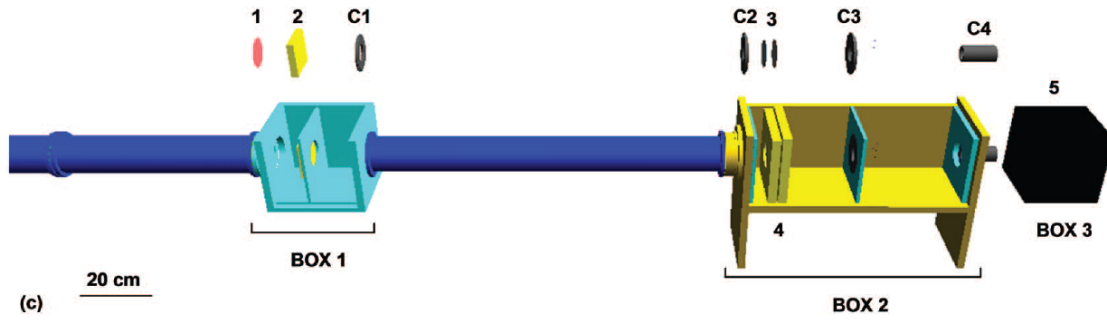
Figure 6.12: MCNPX geometry of the Medicyc beamline elements in the patient room: (1) Kapton vacuum window, (2) range shifter and modulator wheel, (3) mylar foils in the (4) two parallel-plate ionization chambers and (C1-C4) several brass collimators. With permission from (Carnicer et al., 2012).
